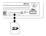
Before removing the SD card, change the radio to another source. To remove, pull straight out.
